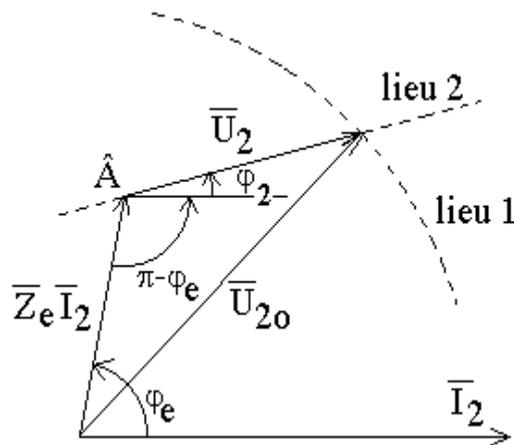
On pose  $Z_e = \sqrt{R_e^2 + X_e^2}$  et  $\varphi_e = \arctg \frac{X_e}{R_e}$
